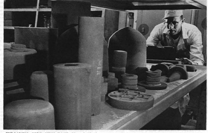
UNLOADING CORE OVEN RACK, Manual Martinez Cores will be placed in molds for next day's schedule checks a typical day's production of sand cores. of pouring. Cores are produced from wooden patterns.
